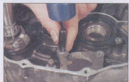
2.13 A sharp tap on the head of a fastener will often break free a corroded thread
