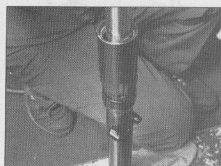
7.16 Install the guide bushing and seal with a driver like this one
