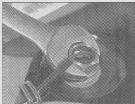
13.6 Disconnect the electrical connector and unscrew the switch from the tank
