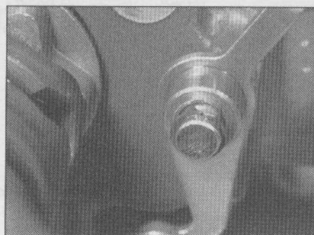
34.5a Remove the snap-ring . . .
