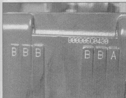
29.12a These marks on the case are bearing size codes . . .
