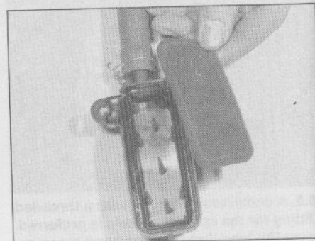
9.4 Remove and clean the foam element
