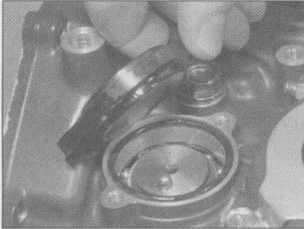
19.5b ... and remove the switch and its O-ring - use a new O-ring during installation
