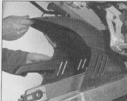
8.3 The rear fender/mudguard on late GSX-R models is attached to the swingarm
