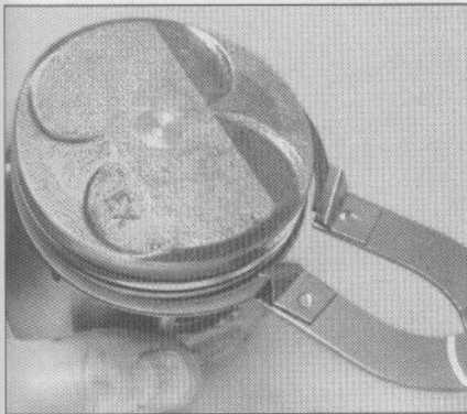
15.6 Remove the piston rings with a ring removal and installation tool
