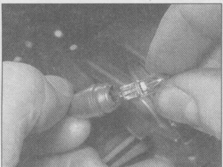
14.1b . . . then pull the bulb out of the socket
