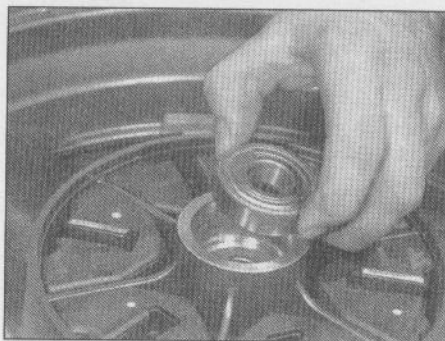
15.13b . . . then install the remaining bearing
