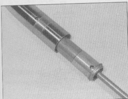
8.75c . . . then pull the cartridge out of the fork tube
