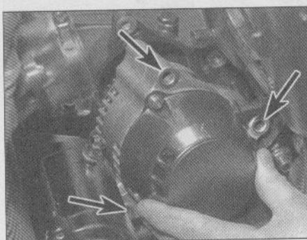
27.7 The alternator is secured by three bolts (arrowed)
