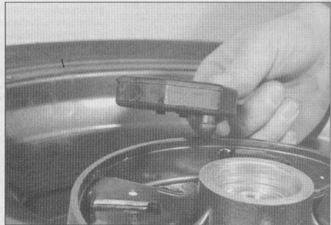
18.3 Pull the damper segments out of the recesses
