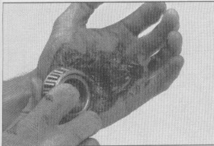
9.23 Work the grease completely into the rollers
