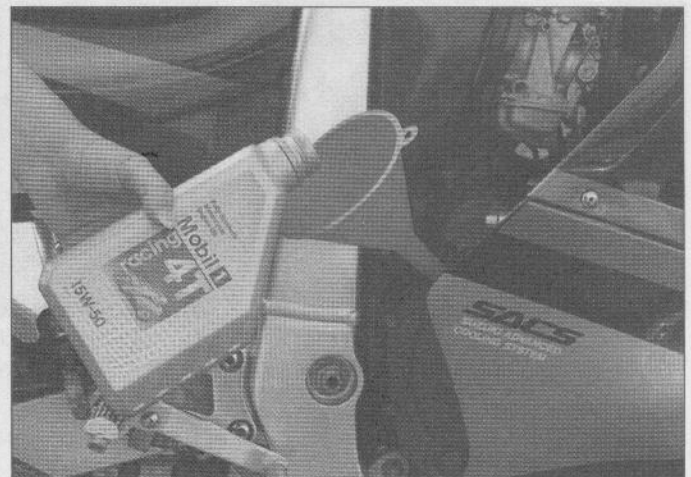
2 If the level is below the Low mark, remove the oil filler cap from the right crankcase cover and add enough oil of the recommended grade and type to bring the level up to the F mark. Do not overfill.
