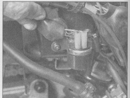
22.1 The starter relay wires are beneath this rubber cover
