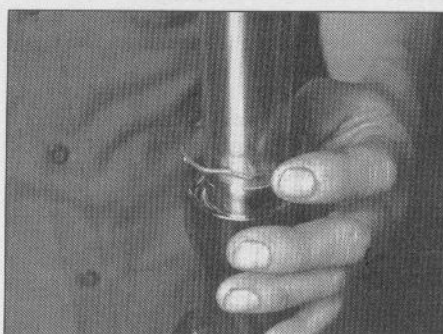
7.8b . . . and slide it off the inner fork tube
