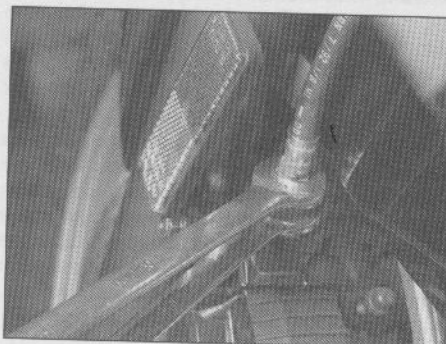
4.2a If the brake line uses a compression fitting, hold the fitting with a backup wrench and undo the line with another wrench
