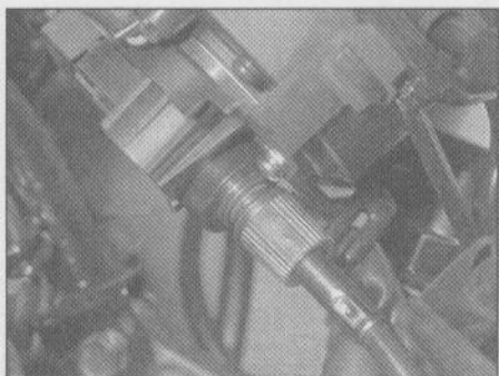
13.18 Disconnect the speedometer cable from the speedometer
