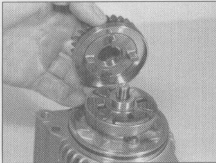
27.11a Lift off the gear and inspect the damper ...
