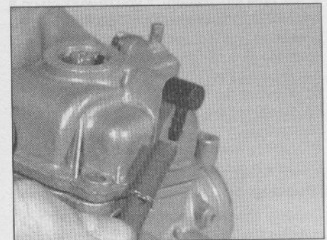
8.58 Disconnect the fuel lines from the carburetors
