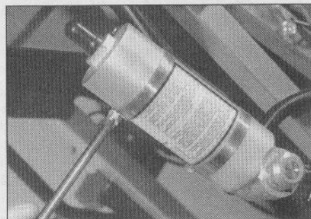
11.3a The remote reservoir is secured by hose clamps below the frame member (GSX-R1100) ...
