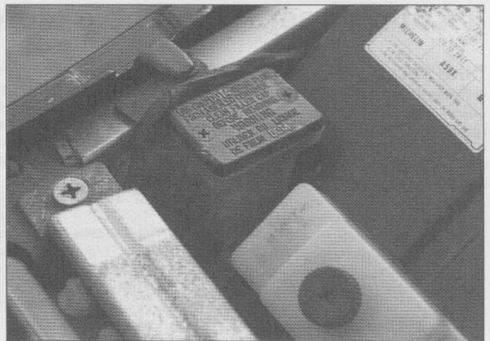
6 The rear reservoir is mounted to the frame. Remove the seat for access.
