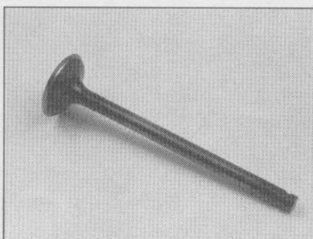
13.17 Check the valve face, stem and keeper groove for signs of wear and damage
