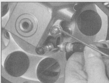
13.19a . . . and from the drive unit on the front fork
