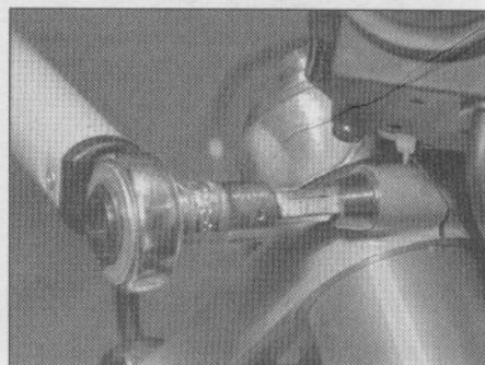
6.9a Remove the upper triple clamp bolts (late GSX-R1100 shown) . . .
