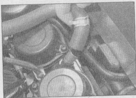
9.2 Loosen the hose clamp and disconnect the breather hose from the air cleaner air box (GSX-R1100 shown, others similar)
