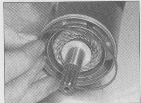
24.5 The large O-ring at each end of the starter housing should be replaced whenever the starter is disassembled
