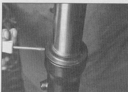
7.7 Pry the dust seal out of the outer tube with a small screwdriver
