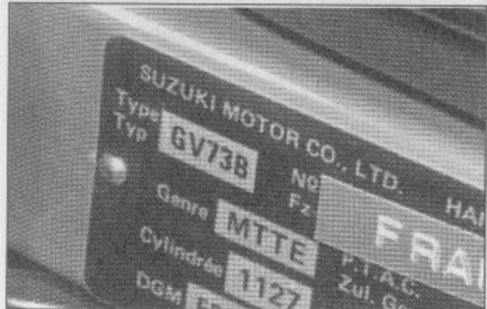
The frame number is stamped on a plate on the left side of the frame ...
