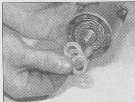
24.4b . . . carefully noting their order so you can reinstall them the same way
