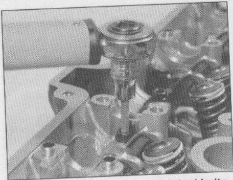
10.41 Tighten the rocker shaft lockbolts
