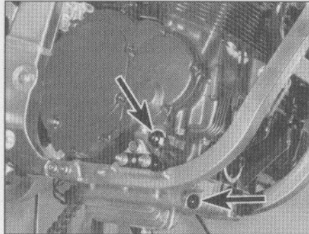
17.6a Unscrew the oil gallery plugs, one on each side of the pan, while the pan is still on the engine (the relief valve and spring are behind the right-hand plug (lower arrow) - the plug in the crankcase (upper arrow) is for checking oil pressure
